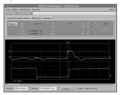
**Summary** By looking at the analog values of a signal as well as the digital values and by correlating the captured data, you can see how software symptoms might be caused by a hardware problem.
